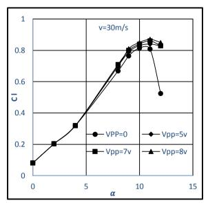
Figure 6.The comparison of computed aerodynamic coefficients experimental data at vpp=0v, 5v, 7v, 8v and f=3.26 kHz at 3%c.
