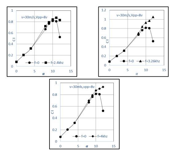
Figure 5. The lift coefficients experimental data with SJA frequency (f=0, 2.4, 3.26 and 4 kHz) are placed at 3% c.
