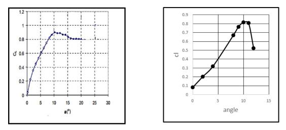
Figure 4. Comparison of experimental data for the lift coefficient over uncontrolled NACA0015 airfoil with the previous experimental data [13, 14]
