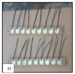
Figure 2. a) synthetic jet actuators arrays
