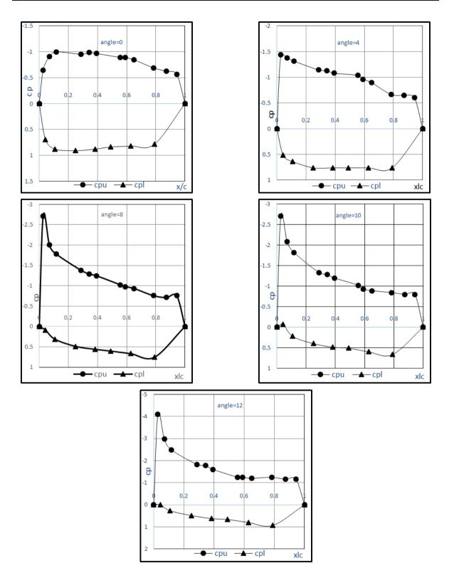
Figure 3. The pressure coefficient curves for the upper (Cpu) and lower surface (Cpl) of the wing
