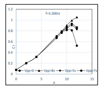
Figure 9. Comparison of lift coefficient at f=3.26 kHz and Vpp = 0, 5, 7 and 8 volts at 6% c.
