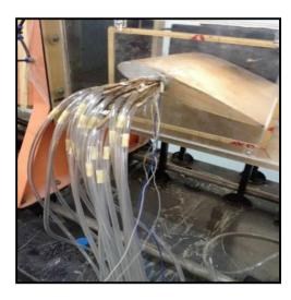
Figure 1.NACA0015 model mounted inside wind tunnel
