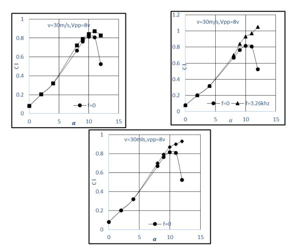
Figure 7. Experimental data of lift coefficients with and without multi-synthetic jets are placed at 6% c at constant Vpp
