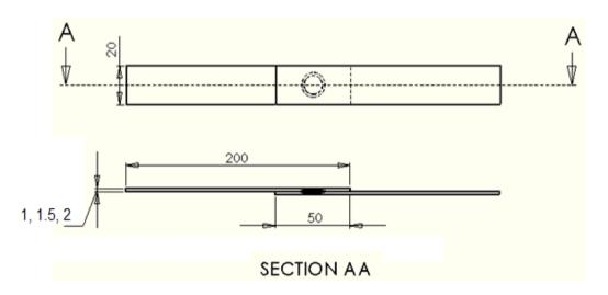
Fig. (2) Dimensions of the steel Sheet specimens
