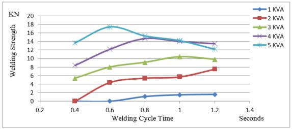
Fig. (5) Relation between welding time and welding strength for sheet thickness (2 mm)
