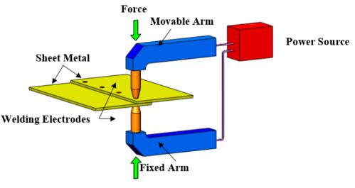
**Force** Fig. (1) Resistance Spot Welding
