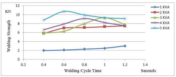
Fig. (4) Relation between welding time and welding strength for sheet thickness (1.5 mm)
