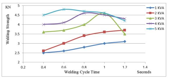
Fig. (3) Relation between welding time and welding strength for sheet thickness (1 mm)
