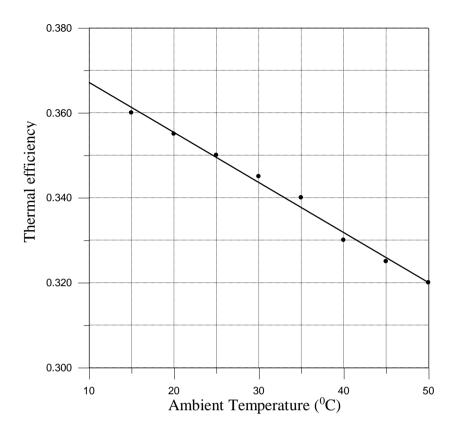
Figure (8): Ambient Temperature versus Thermal efficiency
