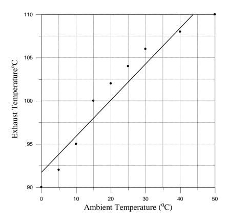
Figure (6): Ambient Temperature versus Exhaust Temperature
