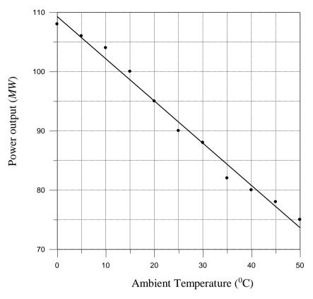
Figure (4): Ambient Temperature versus output Power
