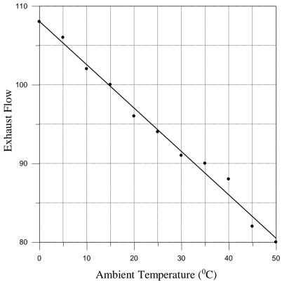
Figure (7): Ambient Temperature versus Exhaust Flow
