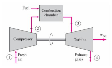
Figure (1): Simple open gas turbine power plant
