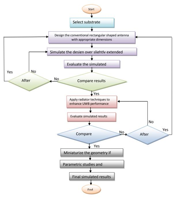
Figure (1): The proposed antennas design methodology.
