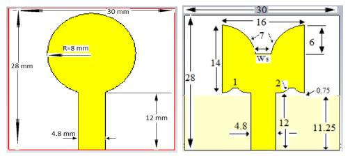
Figure (3): The proposed antenna shapes, (a) circular-shaped patch antenna, (b) as-shaped patch antenna.
