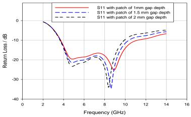
Figure (10): Effects of lower slot depth on  $S_{11}$  for ax-shaped patch antenna.
