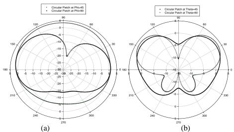
**Figure (5):** Simulated radiation patterns for circular patch form at 8.5 GHz, (a) E-plane and (b) H-plane.
