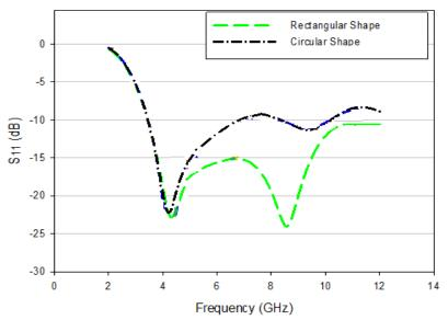
Figure (8): The reflection coefficient for rectangular and circular forms antennas.
