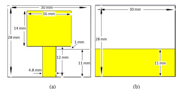
Figure (2): Conventional rectangular-shaped antenna (a) front view, (b) back view.
