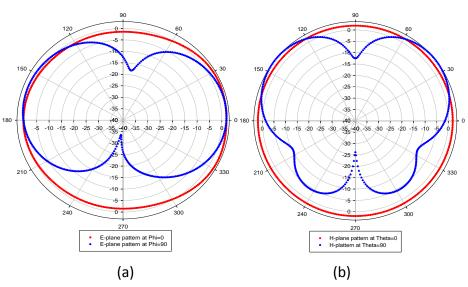
**Figure (7):** Simulated radiation patterns for ax-shaped antenna at resonance frequency of 9 GHz with Phi and Theta equal to 0° and 90° (a) E-plane, (b) H-plane.
