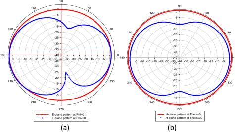
**Figure (6):** Simulated radiation patterns for ax-shaped antenna at resonance frequency of 5 GHz with Phi and Theta equal to 0° and 90° (a) E-plane, (b) H-plane.
