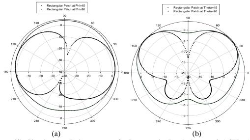
Figure (4): Simulated radiation patterns for Rectangular Patch shape at 8.5 GHz, (a) Eplane, (b) H-plane.
