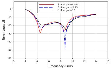
**Figure (9):** Effects of feed gap on  $S_{11}$  for ax-shaped patch antenna.
