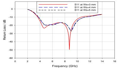
Figure (11): Effects of upper slot width on matching impedance bandwidth for ax-shaped patch antenna.
