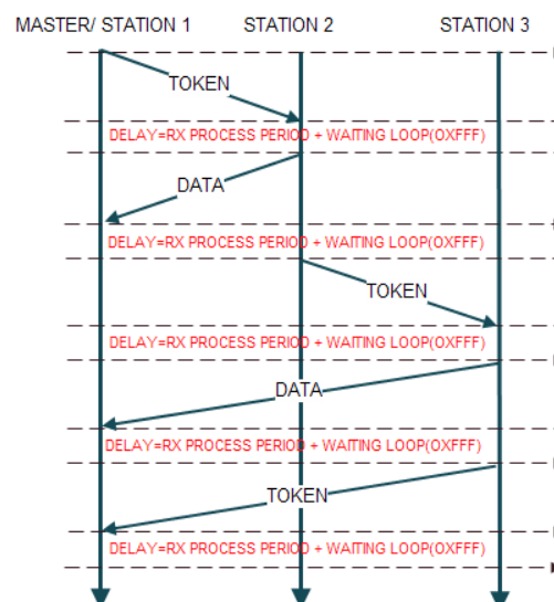
Figure (15): Data and token Flow in RS-485 Bus
