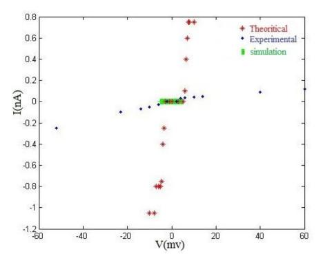
**Figurer (4):** current-voltage curves of single-electron transistor with Fullerene Island for theory and experimental work.
