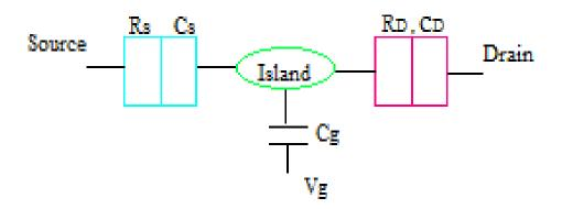
Figure (3): schematic of Single Electron Transistor
