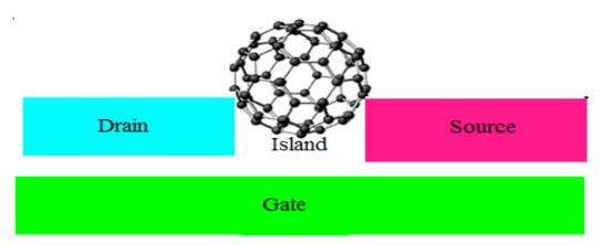
Figure (1): Single Electron Transistor.
