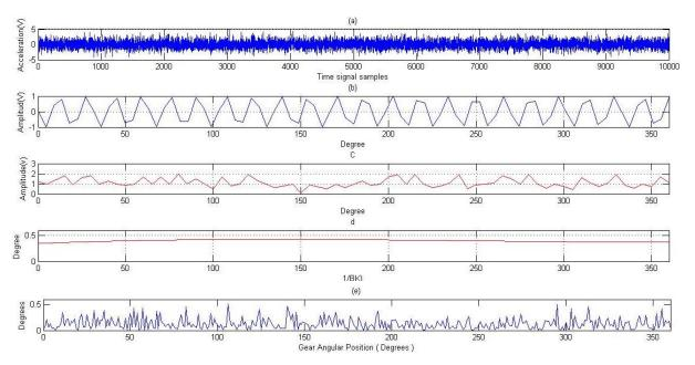
**Figure (4):** Cracked gear processing results: (a) Part of the original vibration signal; (b) Signal average; (c) Wavelet reference function; (d) Beta kurtosis reference function; (e) Phase modulation reference function.
