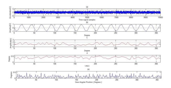
**Figure(3):** Healthy gear processing results : (a) Part of the original vibration signal; (b) Signal average; (c) Wavelet reference function; (d) Beta kurtosis reference function; (e) Phase modulation reference function.
