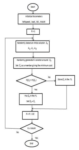
Fig. 8 flow chart of PID-ATS controller
