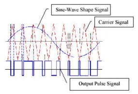
Fig. 3 PWM Signal Synthesis
