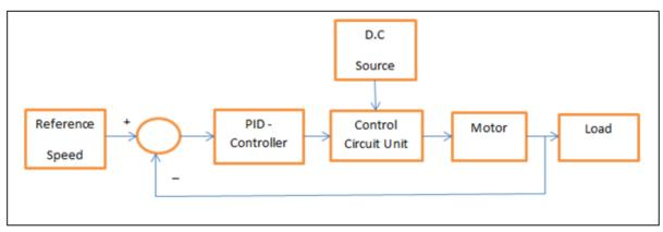
Fig. 5 Block diagram of closed-loop control
