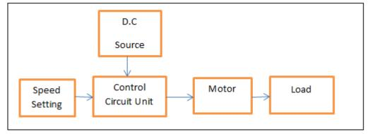
Fig. 4 Block diagram of open-loop control
