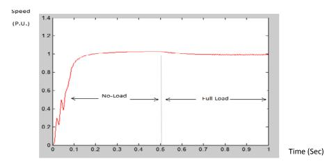
Fig. (11) Speed response of PID Controller tuning parameter using ATS Strategy
