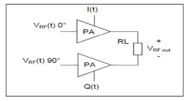
Figure (2): Block diagram of quadrature power amplifier
