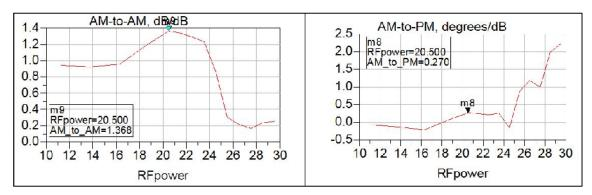
Figure (18): Amplitude distortion (AM-To-AM) and phase distortion (AM-To-PM) of the power amplifier designed at input power is greater than (20dBm)
