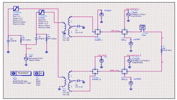
Figure (13): Full schematic design of quadrature power amplifier
