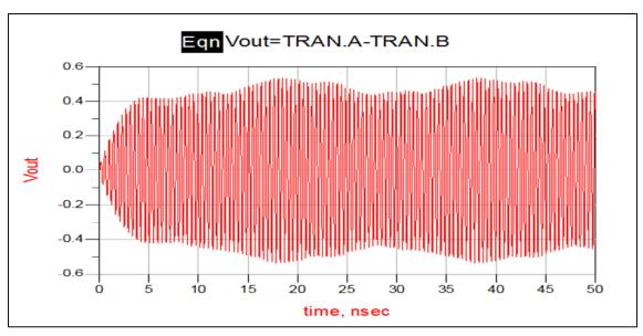
Figure (14): Simulations results for the quadrature power amplifier output with I(t) and Q(t) sinusoid At 50MHz bandwidth
