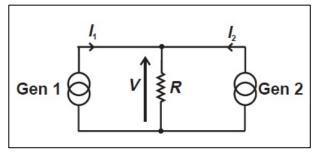
Figure (4): Active load pull schematic
