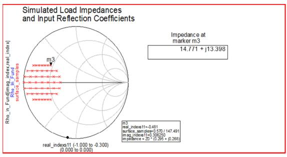
Figure (5): Load pull analysis to determine load impedance for maximum efficiency
