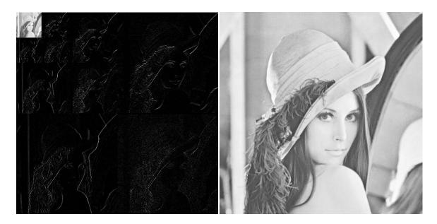
Figure (3): Three-level DHWT decomposition of Lena image and its reconstructed version.
