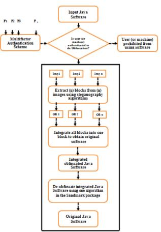
Figure(7): Extraction process of (n) obfuscated software blocks from (n) pre-selected (n) images, scheme1, AODS.
