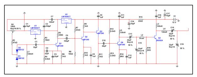
Figure (2): The 416MHz Signal Transmitter.
