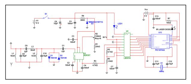
Figure (3): The Electronic Circuit of the Analyzer Module.
