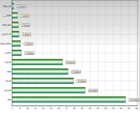
Figuer.10: Procedure Size in the Proposed Algorithm
