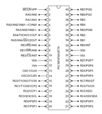
Figuer.4: PIC16F877A Microcontroller
