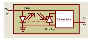
Figuer.2: Remote Sensing Circuit
