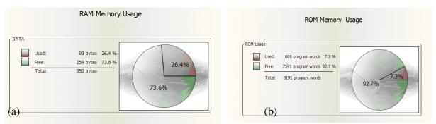
Figuer.9: Memory Graph used in PIC, (a) RAM, (b) ROM
