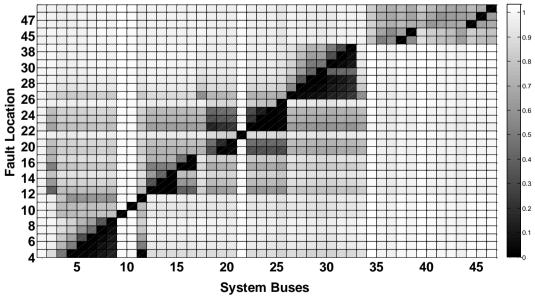
Fig.3 Voltage sag distribution on the system buses attributed to the LLL fault
