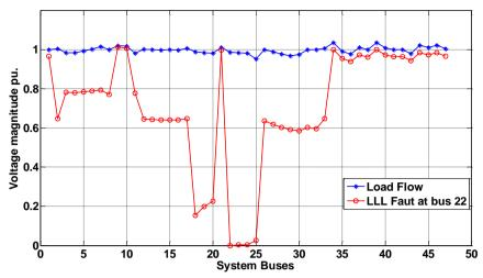
Fig.4 Bus voltage magnitudes before and after LLL fault in Bus 22
