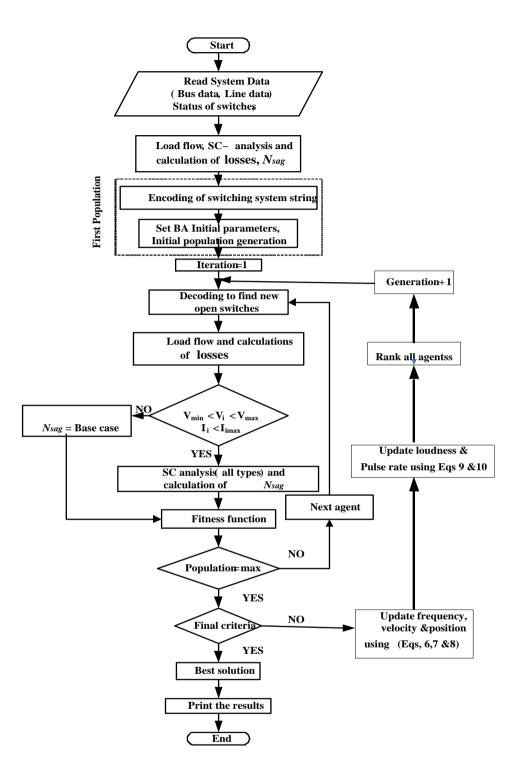
Fig. 1 Flowchart of BA implementation for optimal DNR
