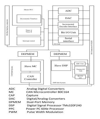
Fig. (6): Block diagram of D-1103 dSPACE
