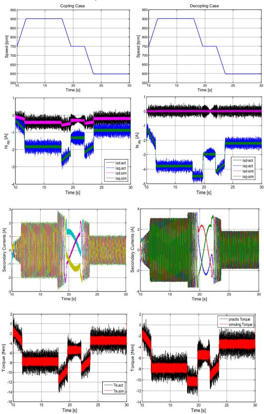
Fig. (7): Secondary d-q currents (upper), Torque and 3PH currents under coupling (left) consequence & decoupling (right).
