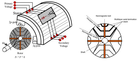
Fig. (1): BDFRM construction (left) Reluctance rotor (right)
