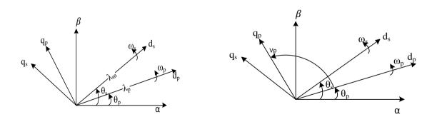
Fig. (2): Reference Frame VC left side FOC right side
