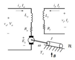
Figure (2). Separately Excited DC motor equivalent circuit.
