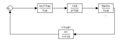
Fig(5): Block model for Speed Controller design
