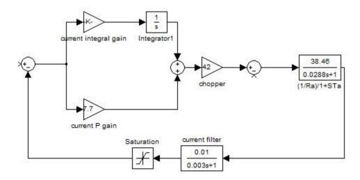
Fig(4): Block Model for Current controller design.
