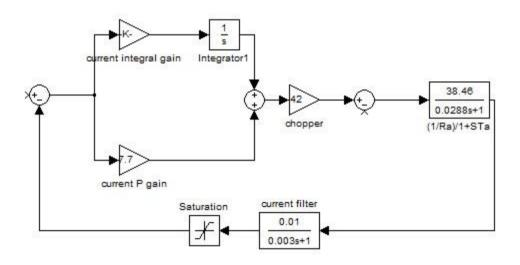
Fig(3):Closed loop system model for speed control of dc motor
