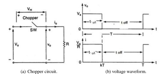
Figure (1) Chopper Circuit and Voltage and Current Waveform
