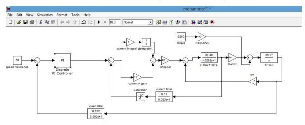
Fig(6): Complete layout for DC motor speed control
