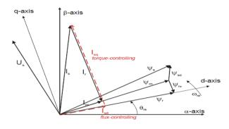
Figure 5. Induction Motor Space-Vector Diagram
