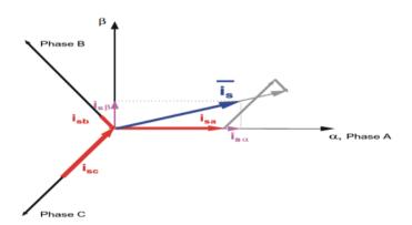
Figure 3. Stator Current Space Vector and Its Projection
