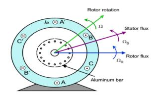
Figure 1. 3-Phase AC Induction Motor
