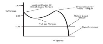
Figure 2. AC Induction Motor Speed-Torque Characteristic
