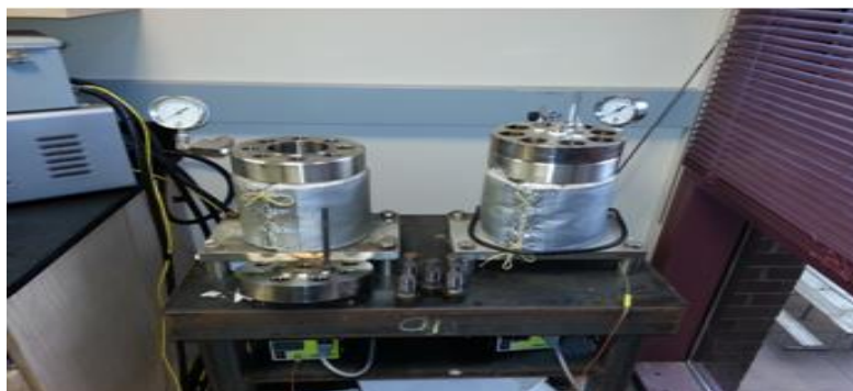
Figure (1) Parr Reactor Autoclave (Home made).
