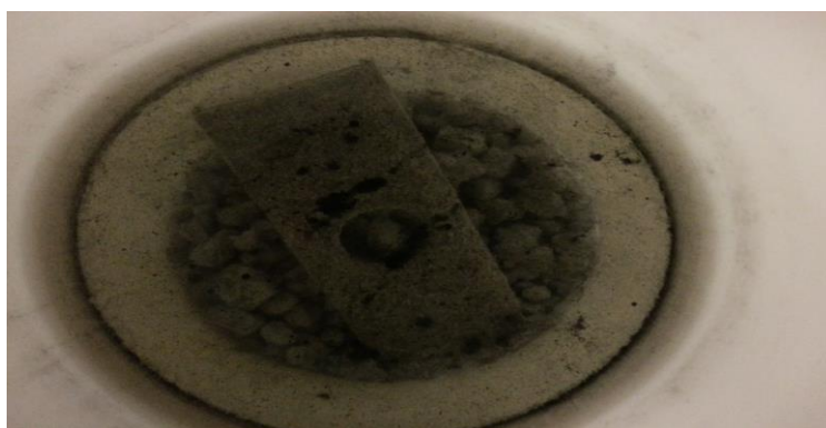
Figure (5) Image of product for TiO 2 /Pd/MWCNTs after removing it from autoclave directly.
