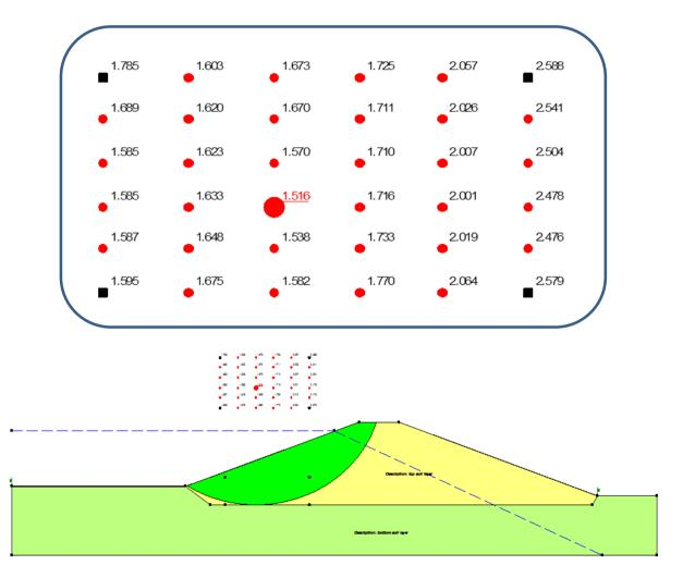
Fig.(2): Al-Fada Dam Case 1-Safety Factor(1) = 1.516
