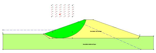
**Fig.(5):** Al-Fada Dam Case 2 -Safety Factor(2) = 1.600
