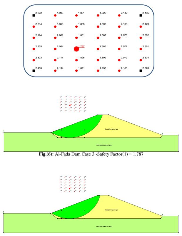
Fig.(7): Al-Fada Dam Case 3 -Safety Factor(2) = 1.828
