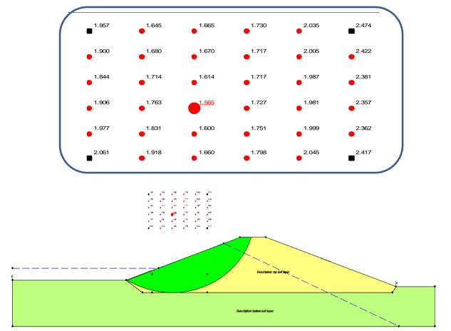
Fig.(3): Al-Fada Dam Case 1 -Safety Factor(2) = 1.538
