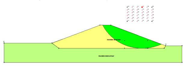
Fig.(9): Al-Fada Dam Case 4 -Safety Factor(2) = 1.931
