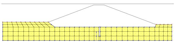
Fig.(10):Finite Element Mesh For foundation of Al-Fada Dam
