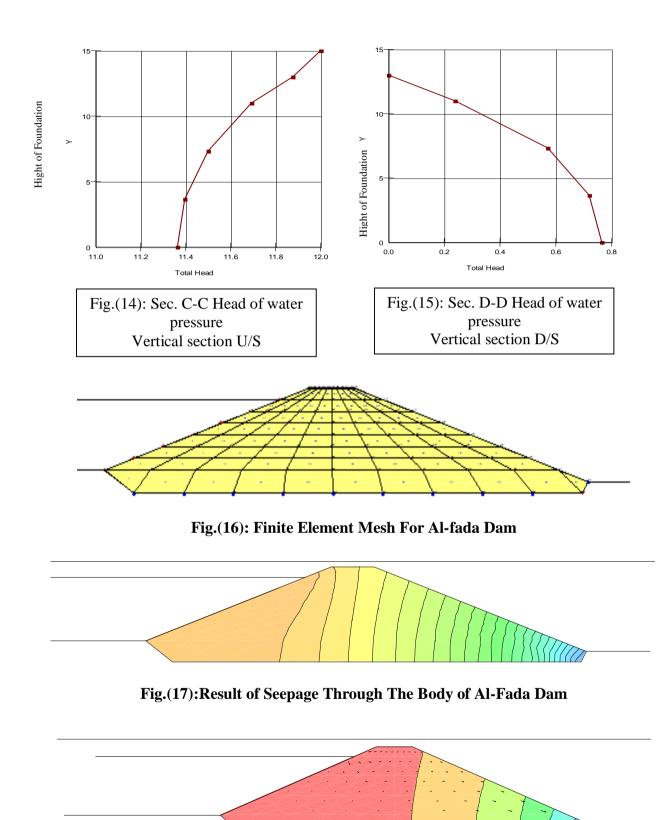
**Fig.(18):Direction of Seepage Through The Body of Al-Fada Dam**
