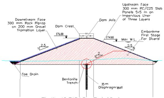
Fig. (1) – AL-FADA Dam Typical Section
