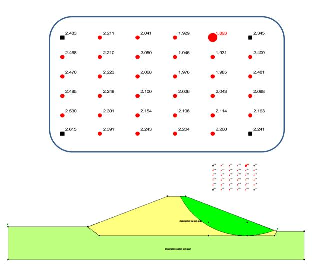
Fig.(8): Al-Fada Dam Case 4 -Safety Factor(1) = 1.893
