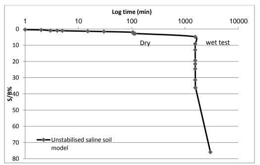
Fig (7): Results of unstabilized saline soil model for natural saline soil brought from Jurf al Milih Region in Diyala Governorate, with10% salinity. Tested at 36.6kN/m<sup>2</sup> applied stress.
