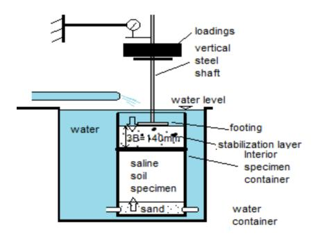
Fig (2): Laboratory model preparation, includes: equipment's, mechanism used for soaking saline soil specimen, and the sand stabilization layer zone.
