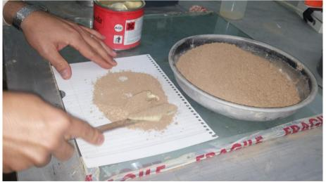
Fig (5): Preparation of sand stabilizing layer, mixed with fly ash and Polyester.
