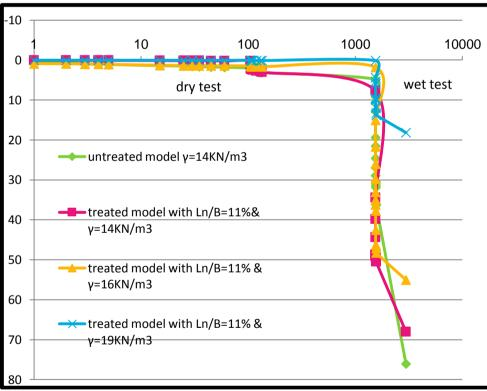
Fig (12) Stabilization of saline soil using a stabilized sand layer, by compaction and the use of 11% randomly distributed waste ferrous material.
