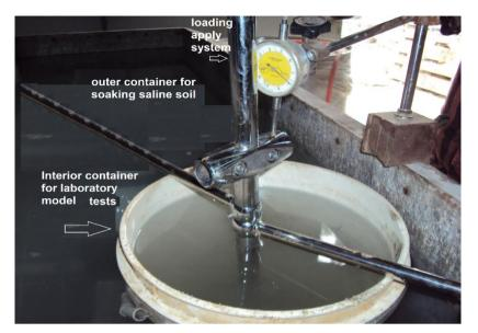
Fig. (3): Model preparation for soaking test for stabilized and unstabilized saline soil by different techniques.
