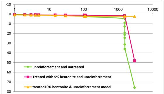
Fig (10): Results of treatment of saline soil by a layer of sand mixed with 5% and 10% Bentonite.
