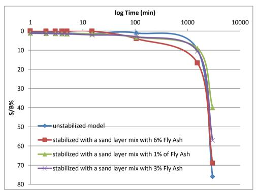
Fig (8): Effect of Fly Ash with Polyester, mix with graded sand layer as a method of saline soil stabilization.
