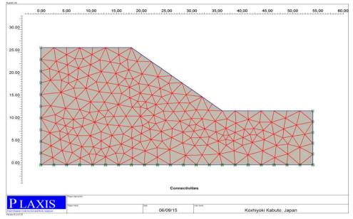
Figure 2. Two Dimensional Finite Element mesh
