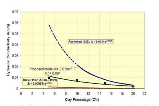
Fig. (4): Comparison between measured of hydraulic and empirical models of (Puckett, 1985) and (Dane, 1992) for different clay percentages.
