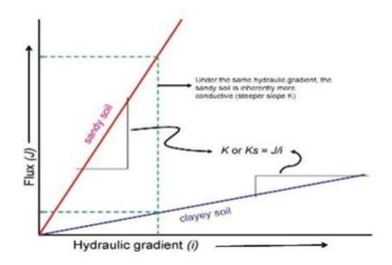
Figure (1): The relationship between flux and hydraulic gradient density.
