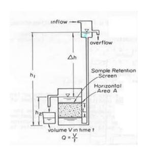
**Figure (2):** Constant head permeameter (After Todd, 1959)
