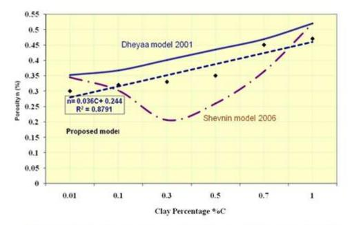
Fig. (3): Comparison between experimental results and empirical models of (Shevnin, 2006) and (Dheya, 2001)
