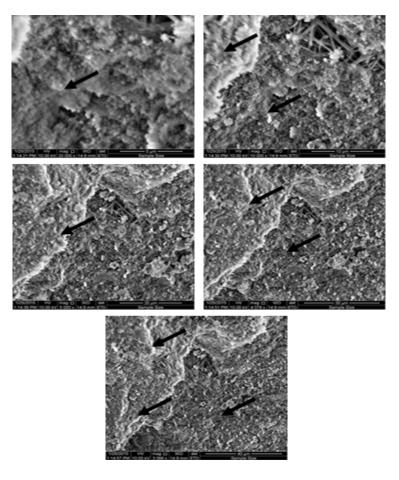
Figure(11). SEM micrographs of the fractured surface of 100% CO<sub>2</sub> cured and 5% fiber/matrix ratio of fiber-cement composites, black arrows indicates denser areas.
