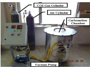
Figure(2). Processing system incorporating CO<sub>2</sub> curing.
