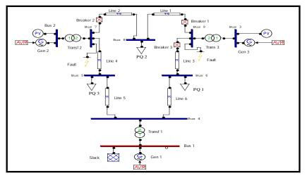
Figure (6) IEEE 3-machine, 9-bus system
