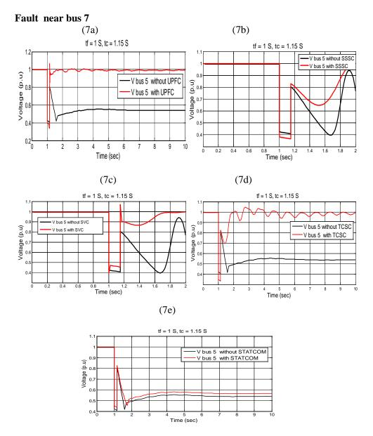
Figure (7a,b,c,d,e)Voltage with and without UPFC,SSSC,STATCOM ,SVC,TCSC
