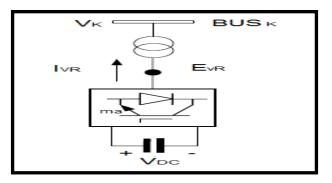
Figure (3) STATCOM Configuration
