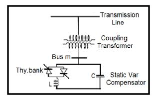
Figure (1) SVC connected to a transmission line
