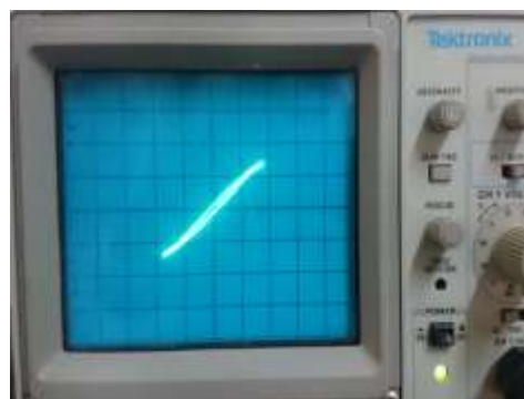
Fig-18 Ballast current waveform and core hysteresis loop at rated current ( 0.43 A )
