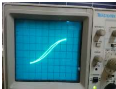
Fig-19 Ballast current waveform and core hysteresis loop at 0.6 A
