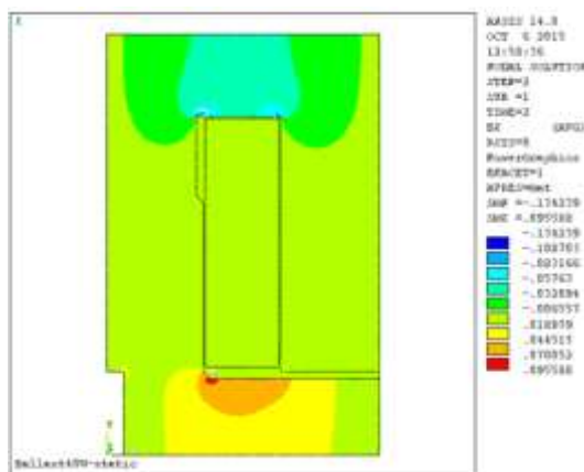
Fig-8 Flux density distribution at rated current
