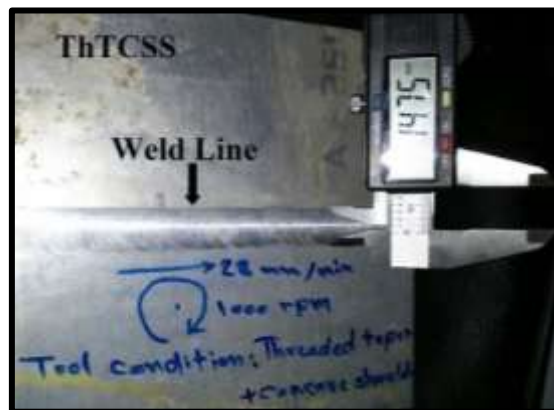
Figure (10): Measurement of weld line dimensions.
