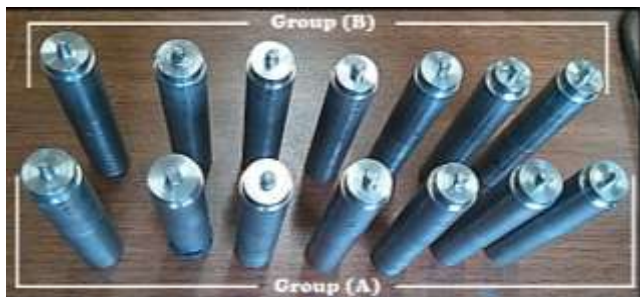
Figure 2: Photograph of FSW tools.
