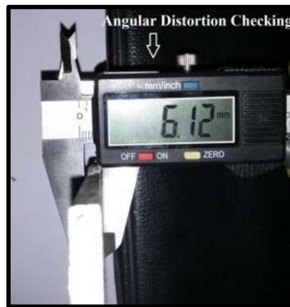
Figure (11): Check of the angular distortion of specimens.
