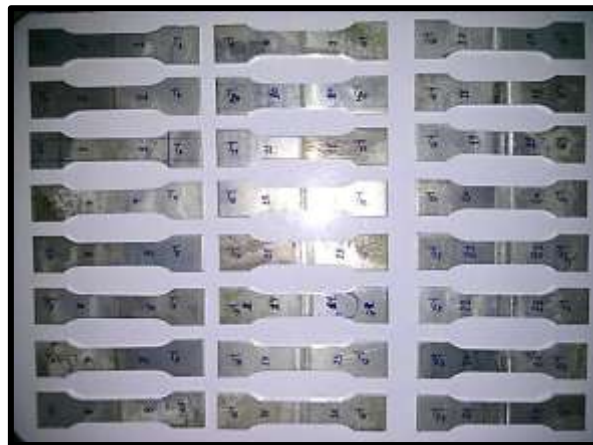
Figure 6 : Tensile test specimens of FSW.
