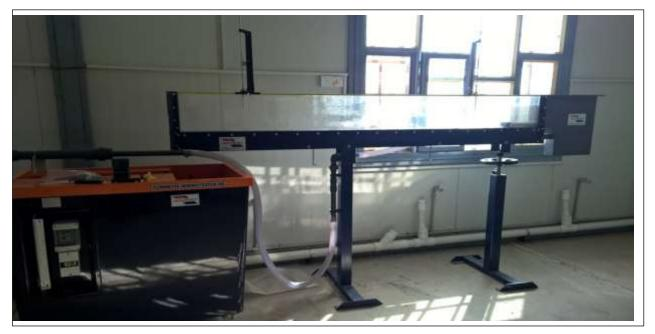
**Fig.(1): The ARMFIELD flume at Al- Qadissiya University / College of Engineering.** For the designing of the models the maximum U/S head above bed channel can be considered 23 cm, and the height of spillways that was 15 cm, so the length of crest is 12 cm. The U/S edge of all spillways can be considered as 1.6 cm which equal to equation 5 to prevent separation of stream flow from the crest. Considering all that nine models at first was designed and made from plywood as in Table (1) below.
