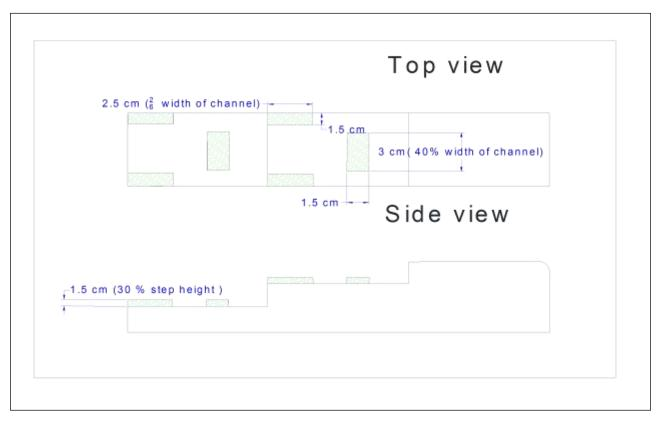
Fig.(9): The dimensions and distribution of blocks in Model No. 11 (case 2).
