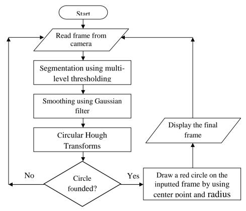
Figure (4): Flow-chart of processing steps
