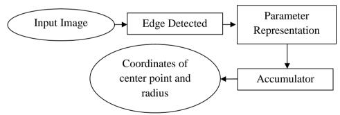
Figure (2): Flow-chart of circular Hough Transform
