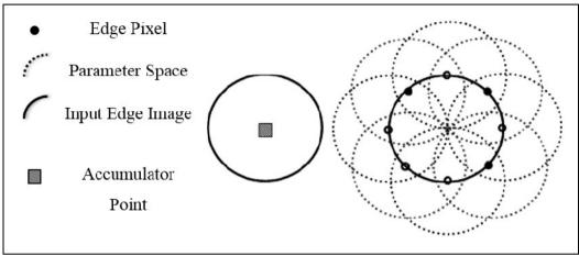
Figure (3): Illustration of circular Hough transform
