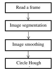
Figure (1): The block diagram of image processing system
