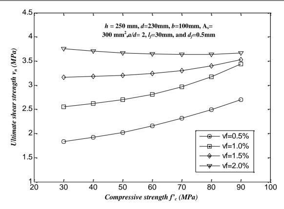
Fig. (6) Effect of  $V_f$  and Compressive Strength on the Shear Strength of FRC Beams without Stirrups.
