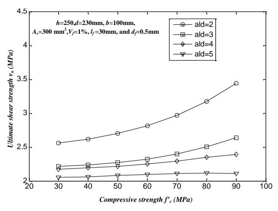
Fig. (3) Effect of a/d and Compressive Strength on the Shear Strength of FRC Beams without Stirrups.
