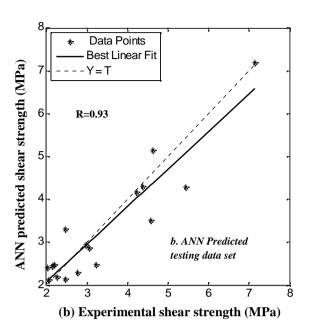
Fig.(2) Comparison of Experimental and Predicted Ultimate Shear Loads: (a) ANN Predicted Training Data Set(b) ANN Predicted Testing Data Set.
