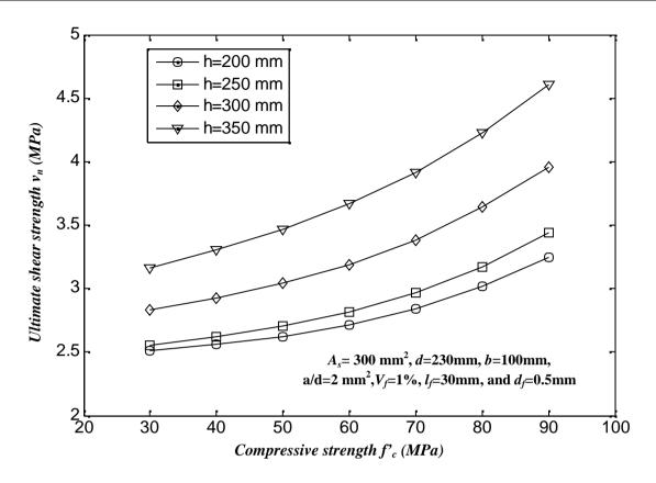
Fig. 5 Effect of Beam Height and Compressive Strength on the Shear Strength of FRC Beams without Stirrups.
