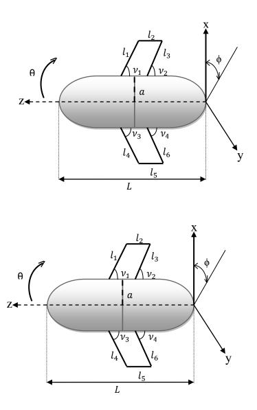
*Fig.*(11): *Geometric shape for missile configuration with wings model,*  $(l_{w1}=l_1+l_2+l_3, l_{w2}=l_4+l_5+l_6, l_1=l_3=l_4=l_6, l_2=l_5 and v_1=v_2=v_3=v_4).$
