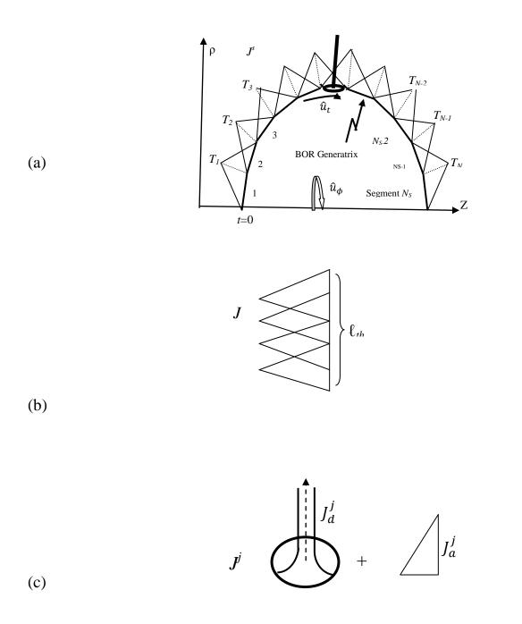
*Fig.(4): Triangular basis functions (a) over the BOR generatrix.(b) on l<sub>th</sub> segment of attachment wire. (c) junction region representation.*
