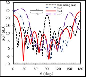
Fig.(13): Backscattered RCS in HP of EFIE-PMCHWT formulation for homogeneous dielectric cylindrical rod with rounded ends of different values of  $\varepsilon_r$ , with two wire-loop wings.
