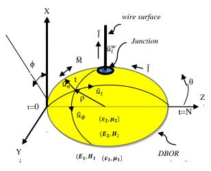
Fig.(1): Homogeneous dielectric object  $(\varepsilon_2, \mu_2)$  embedded in a homogenous medium  $(\varepsilon_1, \mu_1)$  with electric attached wire.  $\overline{J}$  and  $\overline{M}$  are the equivalent surface electric and magnetic currents for the exterior region.
