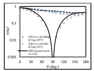
*Fig.(5): Bistatic RCS of dielectric sphere* ( $\varepsilon_r$ =1.44 and radius a=0.159 $\lambda$ ).
