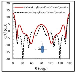
Fig.(10): Backscattered RCS in HP of EFIE-PMCHWT formulation for finite homogeneous dielectric cylinder with two attached wires (radius  $a=0.344\lambda$ ,  $\varepsilon_r=4$ ,  $l_c=1.98\lambda$  and  $l_w=0.880\lambda$ .
