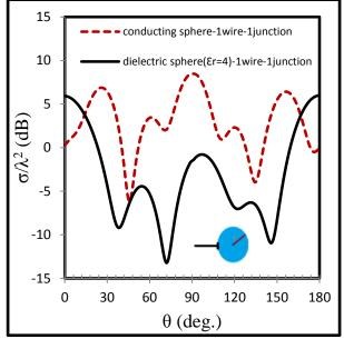
Fig.(9): Backscattered RCS in HP of EFIE-PMCHWT formulation for a homogeneous dielectric sphere with one attached wire (radius  $a=0.159\lambda$ ,  $\varepsilon_r=4$  and  $l_w=0.444\lambda$ .
