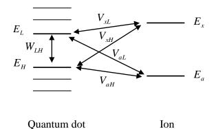
Fig. (1): Energy diagram for ion sputtered from the quantum dot surface
