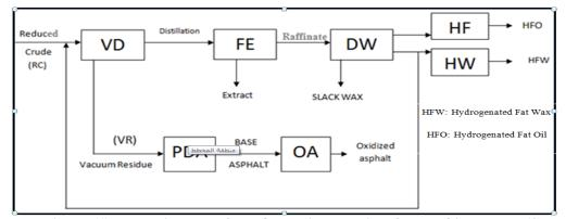
Figure (1) Flow Diagram of the Operational Units of Lube Oil Factory (3)
