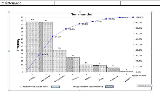
Figure(4) Detailed Frequency of Equipment Failure and Type of Maintenance for ten months
