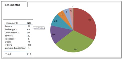
Figure(2) Frequency of Failure Equipment in Lube Oil (3) for ten months.
