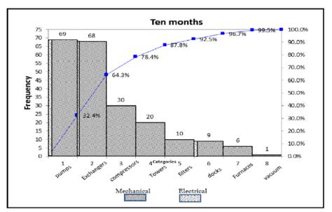
Figure(5) Frequency of Failure either Mechanical or Electrical for ten months
