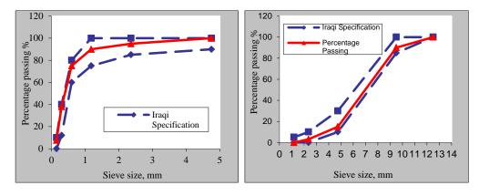
Figure (1):- Grading of fine aggregate Figure (2):- Grading of coarse aggregate
