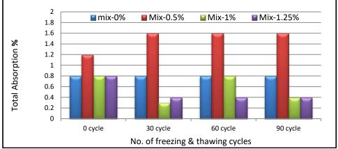
Figure (7):- Percentage of Total Absorption vs. No. of freezing and thawing cycle
