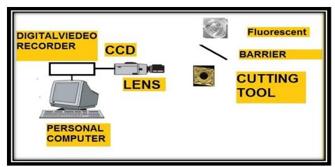
Figure (2). Schematic diagram of the vision based monitoring system. The proposed algorithm
