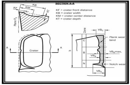
Figure(9) Wear forms in turning (acc. ISO 3685) [11].
