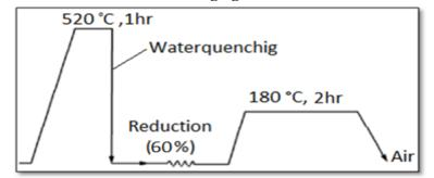
(f) Solution heat treatment at 520 °C /1 hr followed by rolling to (60%) then artificial aging for 2hr.
