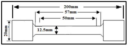
Figure (2). Sample stander depended ASTM- E8 for tensile test.
