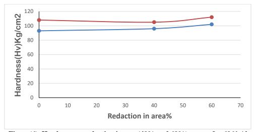
Figure(6). Hardness vs. redaction in area(40% and 60%) curves for 6061 Al alloy, solution heat treated at 520°C for 1hr and aging for ½ hr and 2 hr.
