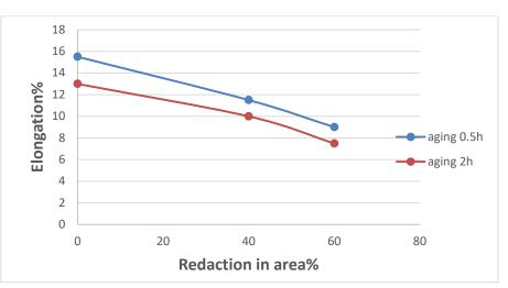
Figure (7). Elongation vs. redaction in area(40% and 60%) curves for 6061 Al alloy, solution heat treated at 520°C for 1hr and aging for ½ hr and 2 hr.
