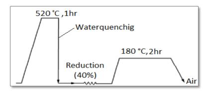
(d) Solution heat treatment at 520 °C /1 hr followed by rolling to (40%) then artificial aging for 2hr.
