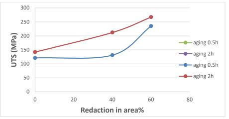
Figure (5). Ultimate tensile strengths vs. redaction in area(40% and 60%) curves for 6061 Al alloy, solution heat treated at  $520^{\circ}$ C for 1hr and aging for  $\frac{1}{2}$  hr and 2 hr.
