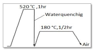
(a) Solution heat treatment at 520 °C /1 hr followed by artificial aging for 1/2 hr.
