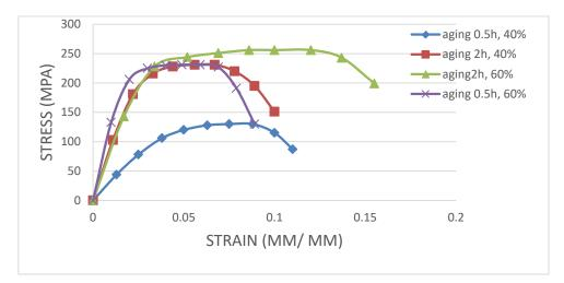
Figure (3). True stress vs. true strain curves for 6061 Al alloy , solution heat treated at 520°C for 1hr with redaction in area (40% and 60%) and aging for (1/2hr and 2 hr).
