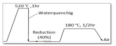
(b) Solution heat treatment at 520 °C /1 hr followed by rolling to (40%) then artificial aging for 1/2hr.
