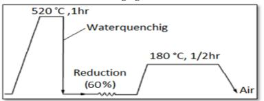
(c) Solution heat treatment at 520 °C /1 hr followed by rolling to (60%) then artificial aging for 1/2hr.
