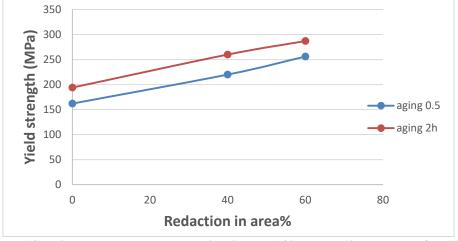
Figure(4). Yield strengths vs. redaction in area(40% and 60%) curves for 6061 Al alloy, solution heat treated at 520°C for 1hr and aging for ½ hr and 2 hr.
