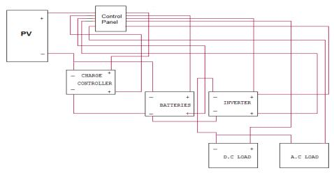
Figure (1): Block Diagram of a Typical Solar System.
