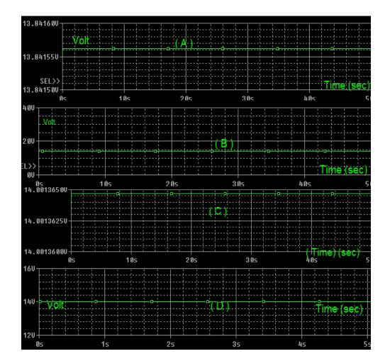
In Figure (8), four traces of the output voltage are simulated with four different input voltage levels at full-load (With  $R_L = 0.1 \Omega$ ).
