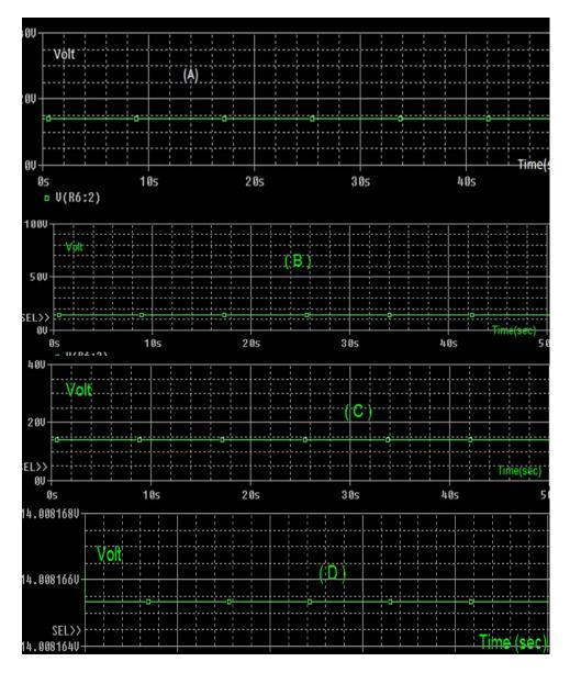
Figure (7): The Simulated Output Voltage of the Charge Controller with Noload at Four Input Voltages.
