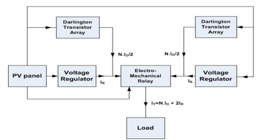
Figure (2): Block Diagram of the Suggested Design of the Charge Controller.
