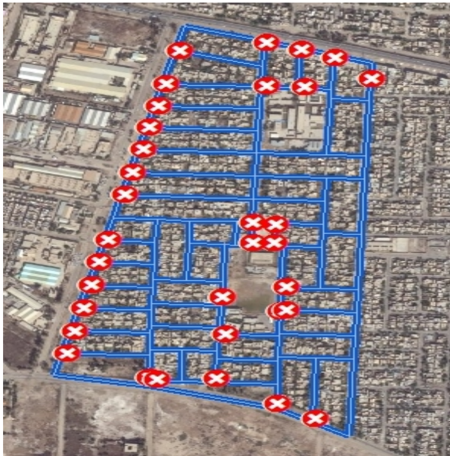
Figure (4). Location of barriers captured by spatial camera . The current optimal route and Barriers
