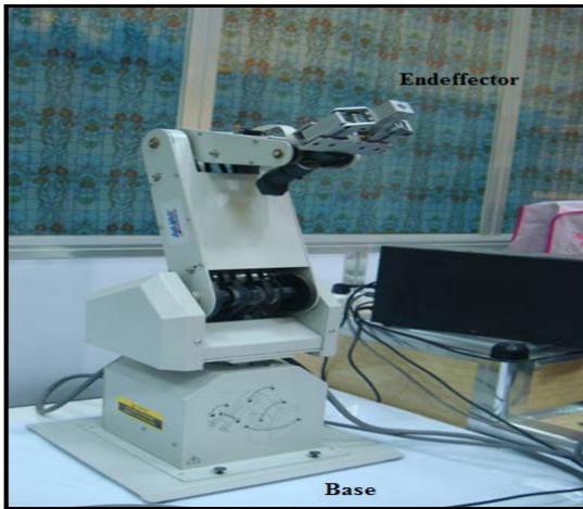
Figure (6)The Lab-Volt Servo Robot System Model 5250(RoboCIM5250)
