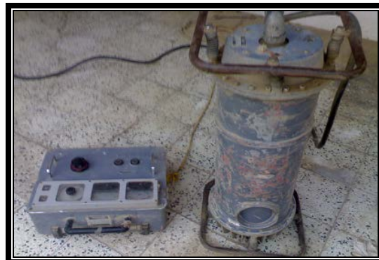
Figure(2) A photograph illustrates the x-ray system
