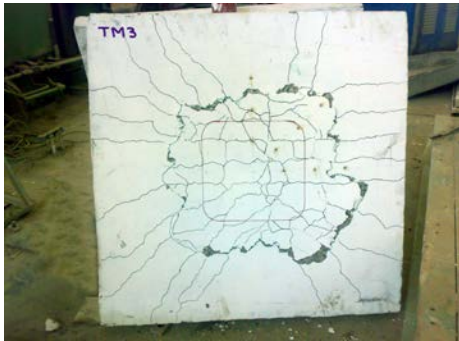
Figure(7) Crack Patterns at Tension Side of Slab R
