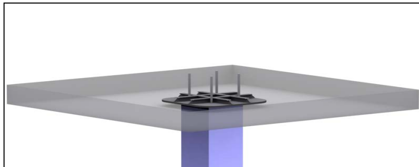
Figure(1) Shearhead Used in the Study
