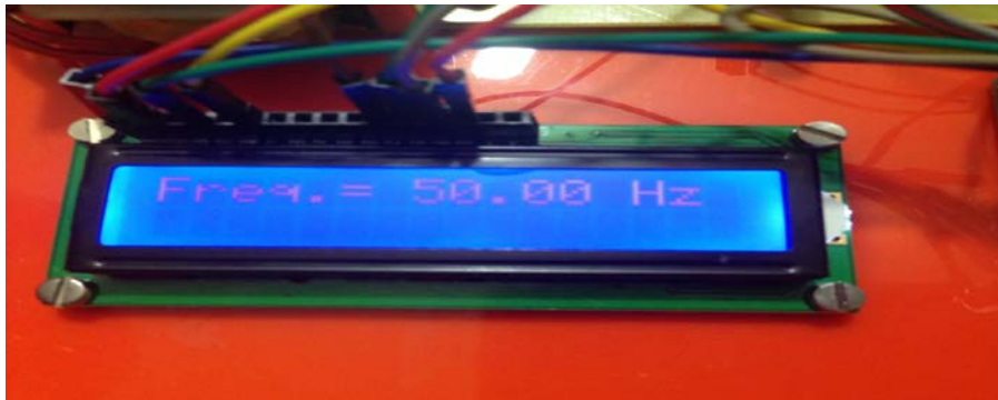
Figure (12): show interfacing LCD with a microcontroller
