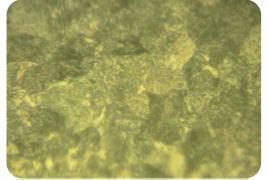
(a) Low carbon steel as received at 500X
