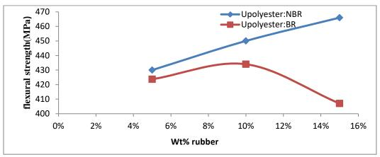
Figure (10) The flexural strength of sherardized low carbon steel as a function of BR or NBR content in the polymer blends coating layer.
