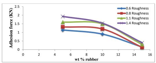
Figure (8) The effect of rubber content on adhesion force for different values of surface roughness (UP : NBR ).
