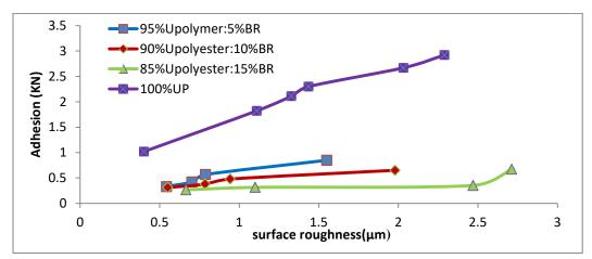
Figure (7) the effect of surface roughness of sherardizing coating on adhesion force for (UP: BR) blend and sherardizing coating low carbon steel.
