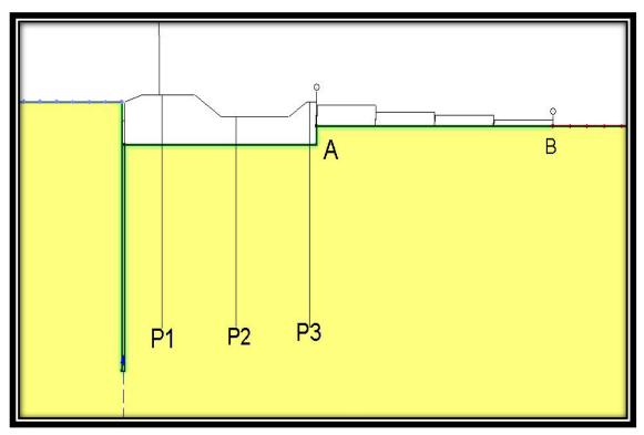
Figure. (1a): profile of allocation the piezometers along the apron
