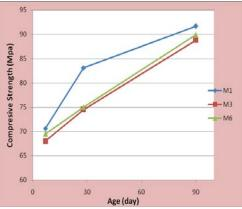
**Figure(1): Development of** compressive strength with age for mixes contain crushed quartzite.
