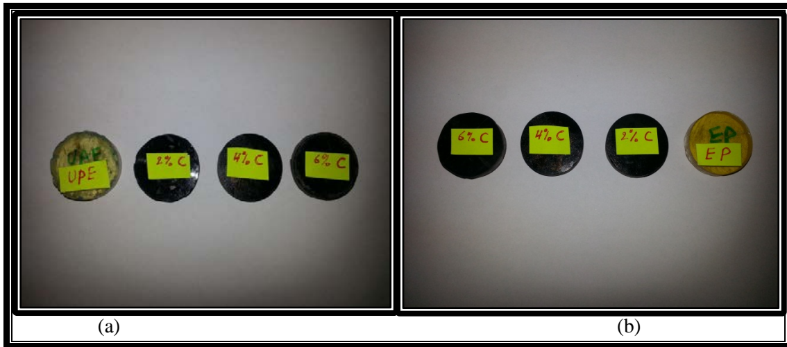
Figure (4): Photograph of thermal conductive test specimens before testing. (a) Pure polyester and TCNP/polyesternanocompositessamples. (b) Pure epoxy and TCNP/epoxynanocompositessamples.
