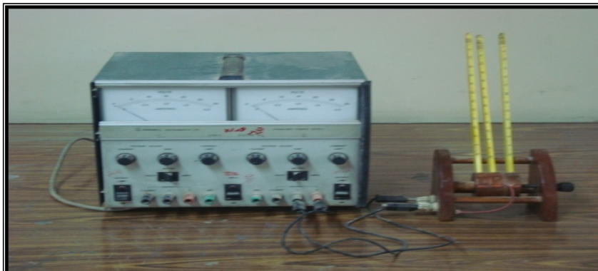
Figure (5): Thermal Conductivity Test Instrument
