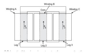
**Fig. (12):** Three-legged core-type transformer.
