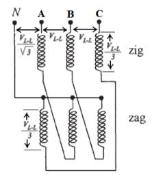
Fig. (3): zig-zag transformer connections.
