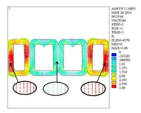
Fig. (20): Zero sequence flux density vectors distribution in iron core.
