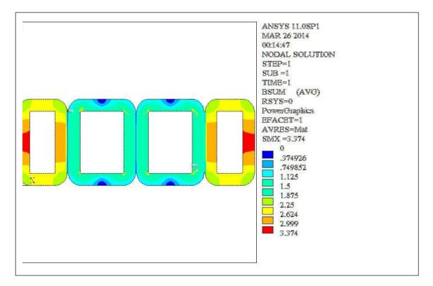
Fig. (21): Contour plot of zero sequence flux density distribution in iron core.
