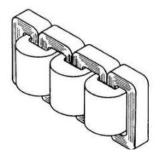
Fig. (14): Five-legged wound core-type transformer.
