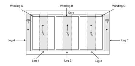
Fig. (15): of five-legged core-type transformer magnetic paths.
