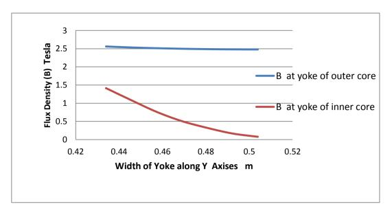
Fig. (24): Illustrated the distribution of magnetic flux at width of yoke region (Y axis) region.
