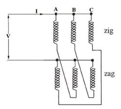
Fig. (17): Connection for Measurement of zero sequence impedance.
