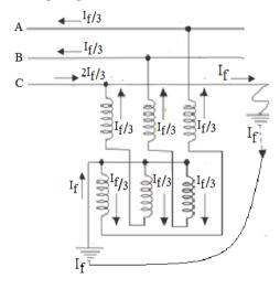
Fig. (5): Earth fault current when single line to ground fault occurs on any phase of the system.
