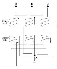
Fig. (2): zig-zag transformer arrangement.
