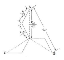
**Fig. (4):** Vector diagram of a zig-zag transformer connection.
