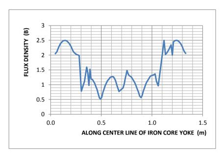
Fig. (23): Illustrated the distribution of magnetic flux along the center line of X direction (length of core) at yoke region.
