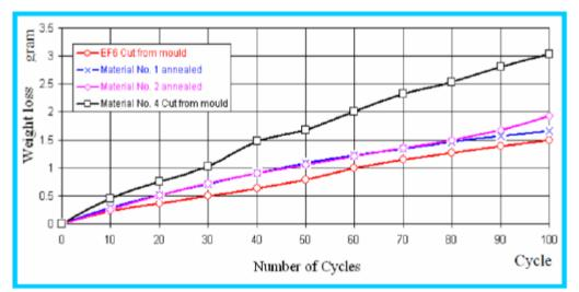
Figure (14): Average Weight loss of material No. 4 (as-cast condition) compared with other (heat treated condition) materials as a function of number of cycles tested at 850°C.
