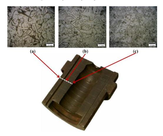
**Figure (3):** Microstructure of material EF6 (Sun quick glass blow mould provided by OMCO – a Belgium company) taken in three locations (a = by the outside of the mould wall), (b = in the mid thickness of the mould) & (c = by the cavity of the mould).
