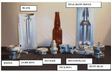
Figure (1): Glass blow mould parts <sup>(13)</sup>.
