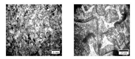
Figure (5): Microstructure of material no. 4 (as cast condition without heat treatment).
