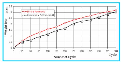
Figure (13): Average Weight loss of material No. 4 compared with EF6 material as a function of number of cycles for as-cast condition tested at 600°C.
