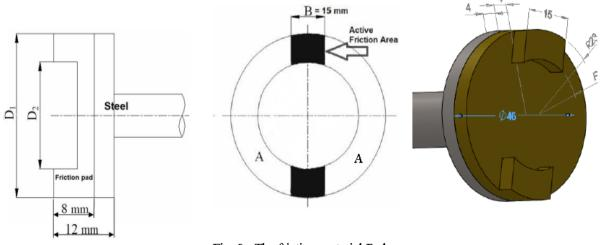
Fig. 8. The friction material Pad
