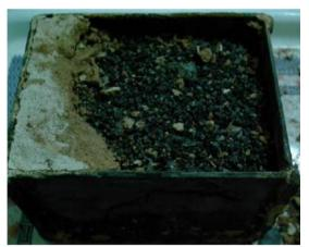
Figure (2): specimens packing sealed steel box.
