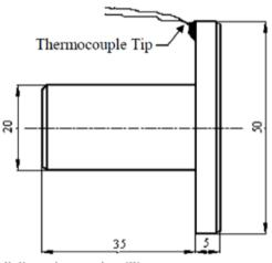
All dimensions are in millimeters Figure (7): wear test specimens (for both as cast & heat treated condition).
