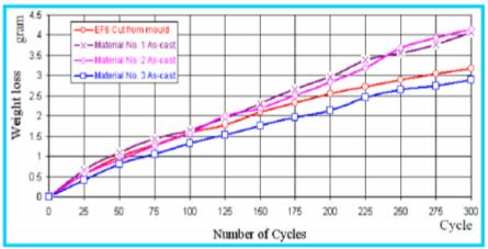
Figure (9): Average Weight loss (gram) as a function of number of cycles for as-cast materials (Before annealing) tested at 600°C.
