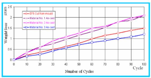
Figure (11): Average Weight loss (gram) as a function of number of cycles for as-cast materials (Before annealing) tested at 850°C.
