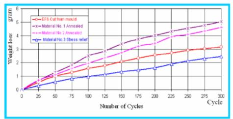
Figure (10): Average Weight loss (gram) as a function of number of cycles for heat treated materials (After full annealing) tested at 600°C.
