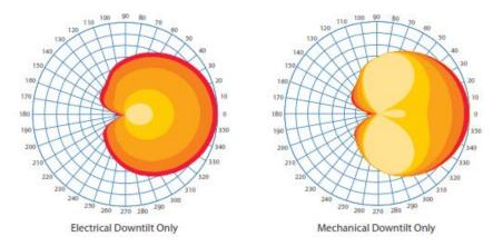
Figure (3): Electrical versus mechanical down tilt angle comparison
