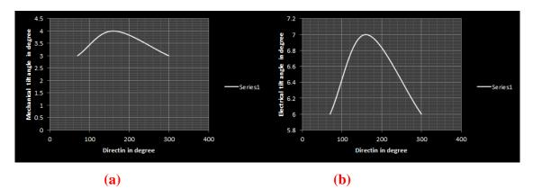
Figure (9) (a): The mechanical tilt angle versus the direction for Bakhtiary site.(b): The electrical tilt angle versus the direction for Bakhtiary site.
