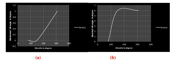
Figure (8) (a): The mechanical tilt angle versus the direction for Salim site.(b): The electrical tilt angle versus the direction sites for Salim site.
