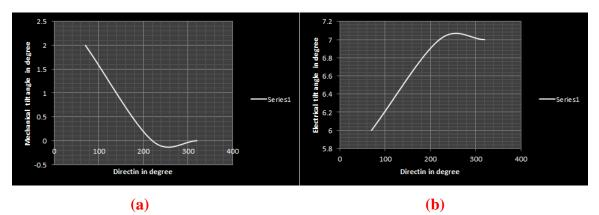
Figure (6) (a): The mechanical tilt angle versus the direction for Ashty new site.(b): The electrical tilt angle versus the direction for Ashty new site.
