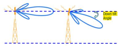
Figure (4): Mechanical down tilt versus electrical down tilt
