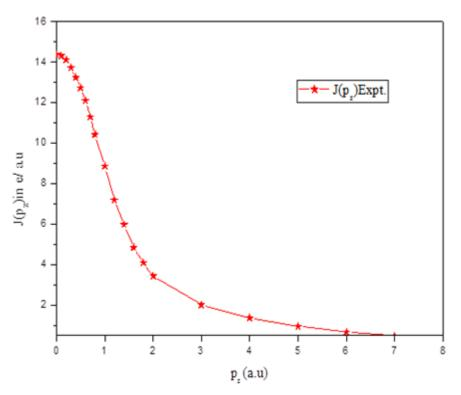
**Figure (1):** Experimental Compton profile of CaCl<sub>2</sub>. The profile is convoluted with the Gaussian of 0.6 a.u. FHWM.
