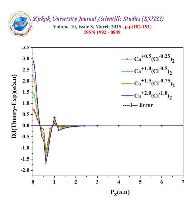
**Figure (2):** The difference ( $\Delta J$ ) between convoluted ionic model and experimental Compton profiles of CaCl<sub>2</sub>. Experimental error( $\pm \sigma$ ) are also shown at points. All ionic profile are convoluted with Gaussian of 0.55 a.u.
