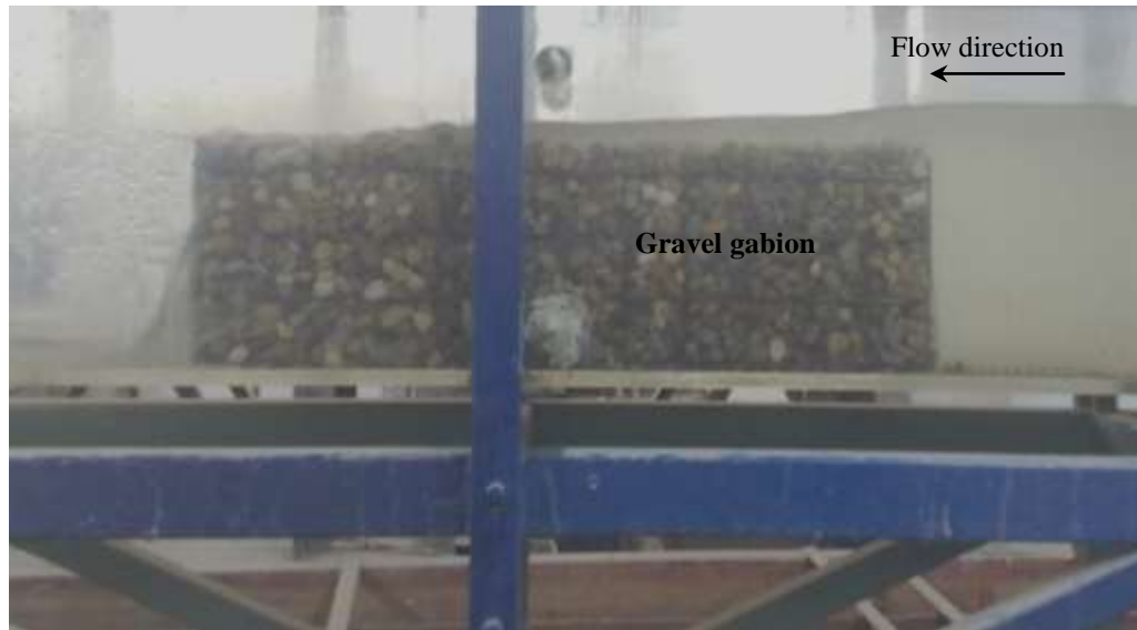
Figure 5. View of gabion weir used in the study.
